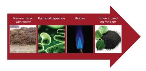
complete the process is called retention time. As the matter flows through the tank, biogas begins to accumulate in the upper part of the digester. This gas can be transported to the kitchen by a hose or pipe fitted with a valve, or it can be stored in a separate plastic container.
