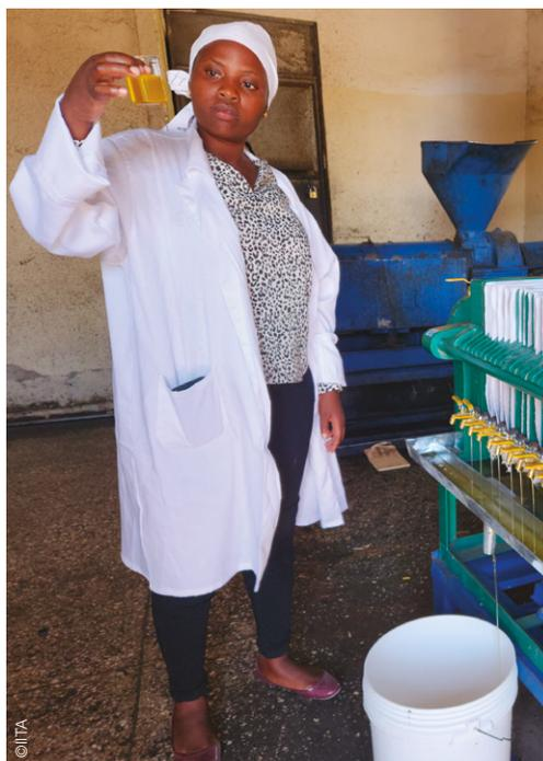
Project beneficiary working with a sunflower oil press and filtering machine. The new equipment allows for quick processing of small quantities of oil for local farmers.
